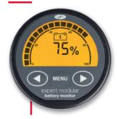
Standard view The image above shows the normal operating mode with the second parameter row disabled. This results in a clean display area that only shows the battery state of charge (%) and the bar graph. A perfect mode for less technical end users.
